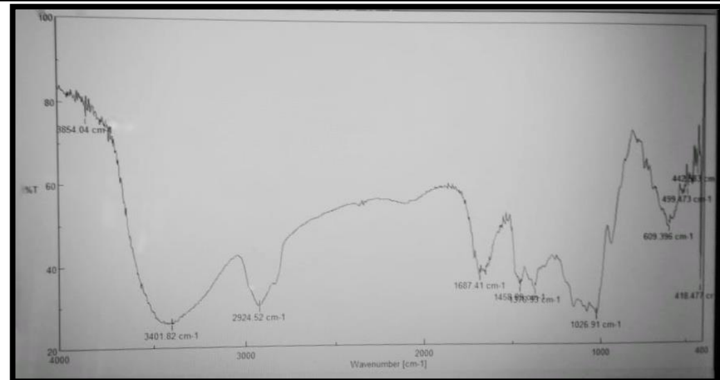
Fig. 3. FTIR Spectrum of the physical mixture of Dexamethasone, Metronidazole, Carbopol 940 and Xanthan gum
