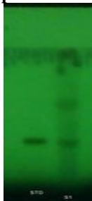
Figure 4. HPTLC plate at 254 nm showing STD and sample at 0 th month
