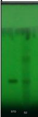
Figure 8. HPTLC plate at 254 nm showing STD and sample at 6th month
